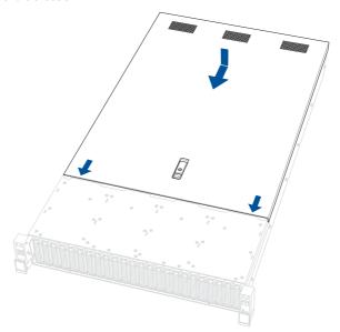
2. Push the latch downwards to lock the chassis cover into place.
