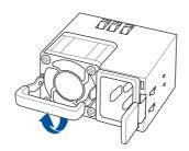
2. Hold the PSU lever and press the PSU latch inwards, then carefully pull the PSU out of the system chassis.
