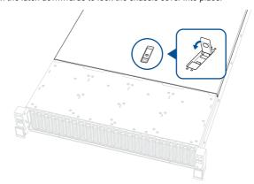
3. Turn the screw clockwise to lock the latch.
