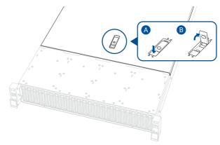
3. Slide the chassis cover towards the rear of the chassis, then lift and remove it from the chassis.
