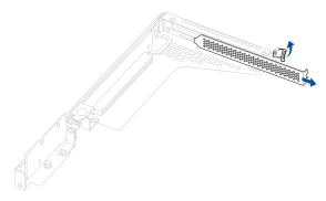
Install the expansion card, then push the slot cover lock inwards to secure the expansion card.
