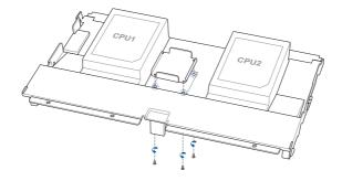
2. Install the cache vault power module, then connect the cache vault power module to the HBA/RAID card.
