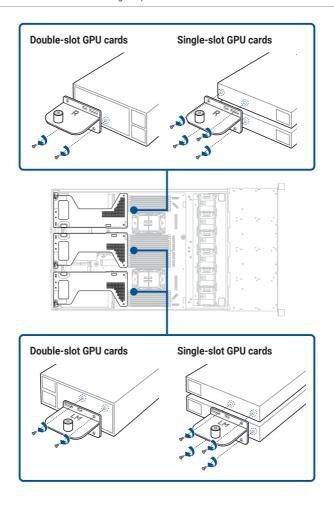
6. Install the expansion card bracket, then connect the GPU power cable to the GPU card.
