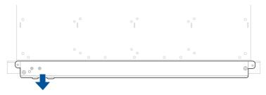
3. Slide the bezel towards the left and remove it from the chassis.
