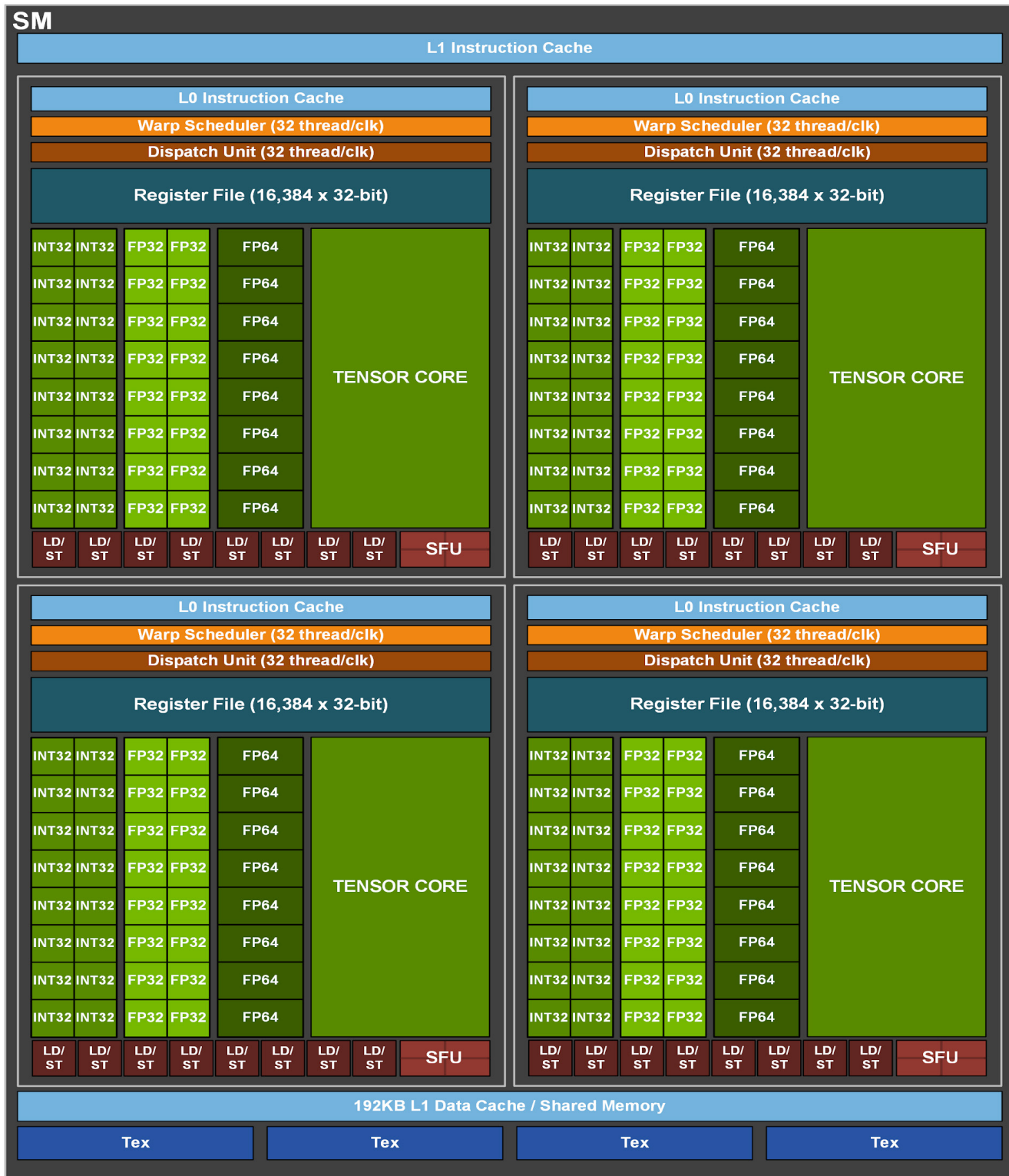
Figure 7. GA100 Streaming Multiprocessor (SM)
