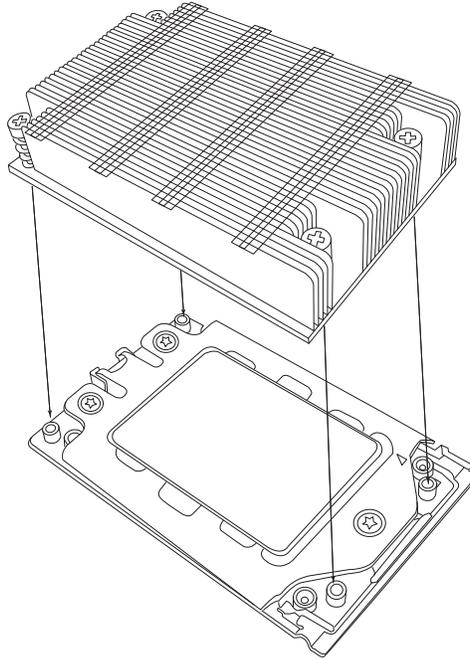
12. Using a diagonal pattern, tighten the four screws down on the heatsink in a clockwise fashion till it is secure. The heatsink will now be secured and you have finished installing the processor and heatsink onto the motherboard. Repeat this procedure for any remaining CPU sockets on the motherboard.
