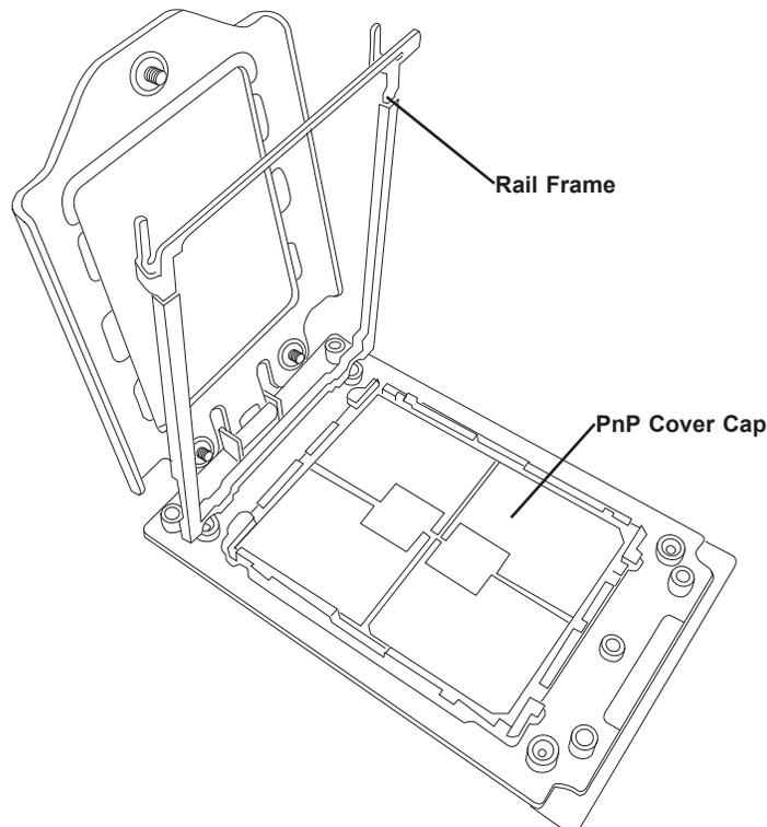
4. Remove the external cap from the Rail Frame by pulling it upwards through the rail guides on the rail frame.
