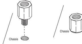
3. Locate the matching mounting holes on the chassis. Align the mounting holes on the motherboard with the mounting holes on the chassis.
