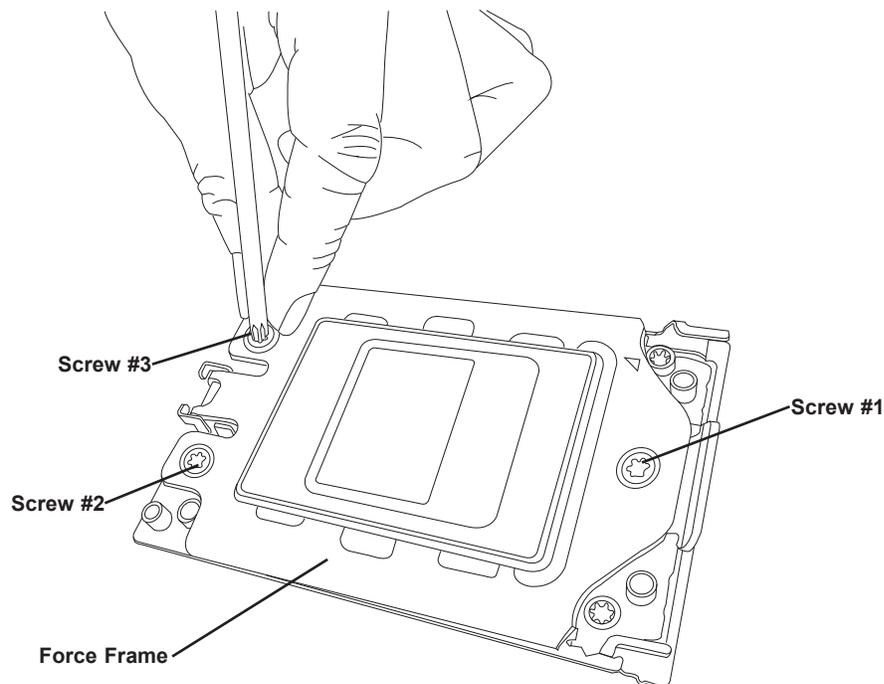
2. The spring-loaded force frame will raise up after the last screw securing it (#1) is removed. Gently allow it to lift up to its stopping position.
