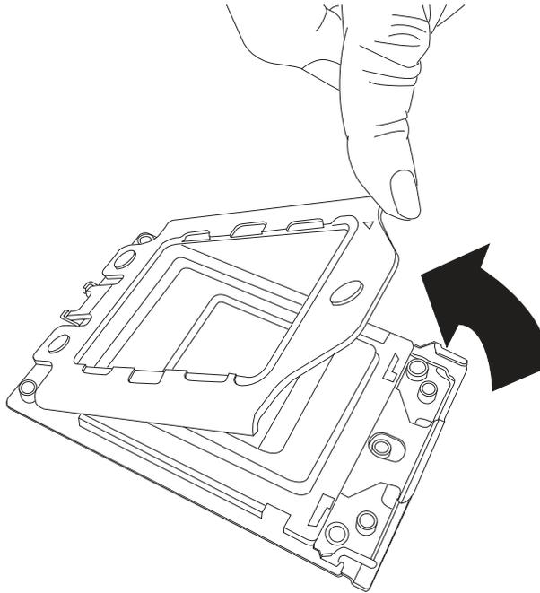
3. Lift the rail frame up by gripping the lift tabs near the front end of the rail frame. While keeping a secure grip of the rail frame, lift it to a position so you can do the next step of removing the external cap.
