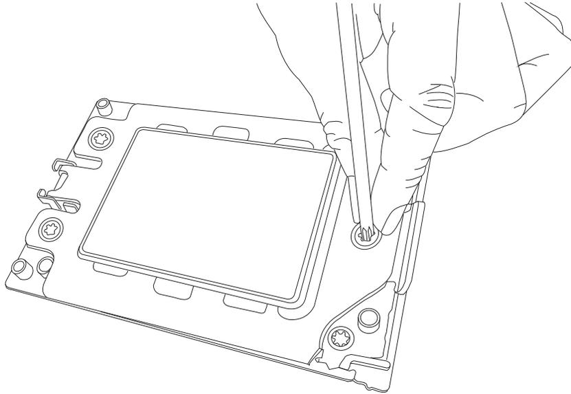
10. Place and re-screw the screws in the reverse order to the way you removed them (holes 1-2-3 in order). When finished, the force frame will be secure over both the rail frame and CPU package.
