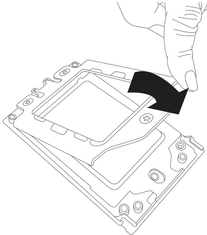
8. Gently lower the rail frame down onto the socket until the latches on the rail frame engage with the socket housing and it rests in place. **DO NOT** force it into place!
