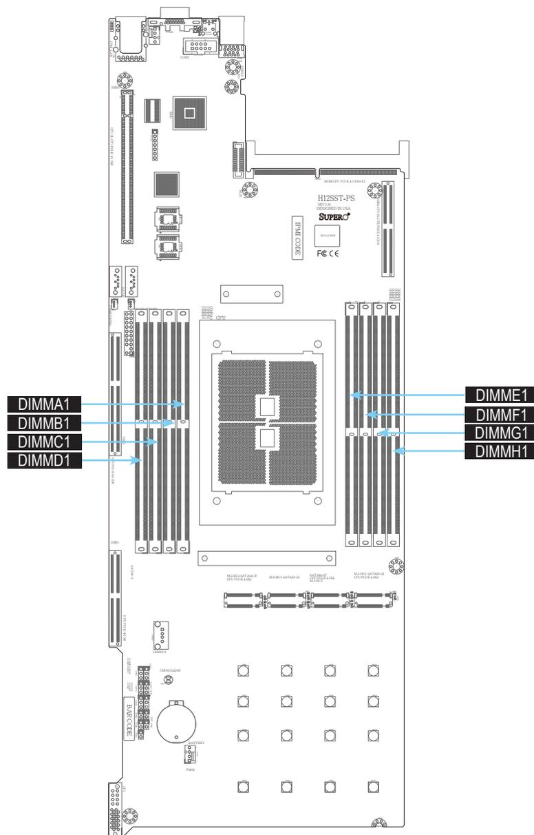
Figure 2-2. DIMM Numbering
