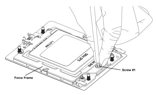
2. The spring-loaded force frame will raise up after the screw securing it (#1) is removed. Gently allow it to lift up to its stopping position.
