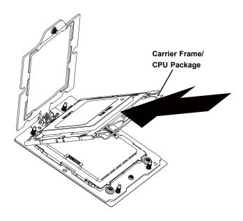
**Note:** You can only install the CPU inside the socket in one direction with the handle at the top. Make sure that it is properly inserted into the CPU socket before closing the rail frame plate. If it doesn't close properly, do not force it as it may damage your CPU. Instead, open the rail frame plate again, and double-check that the CPU is aligned properly.
