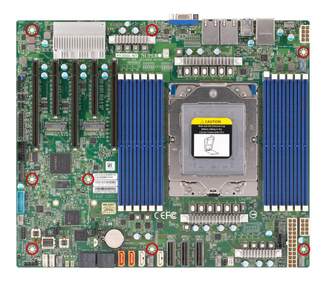
Figure 2-1. Motherboard Mounting Holes
