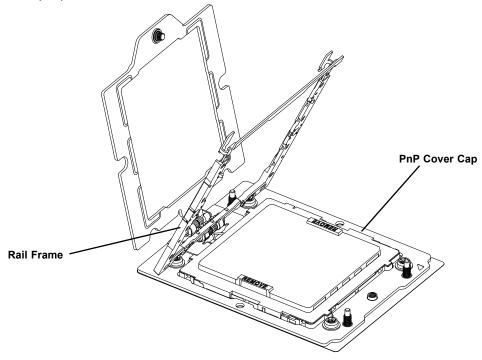
4. Remove the external cap from the rail frame by pulling it upwards through the rail guides on the rail frame.
