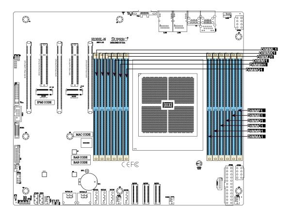
Figure 2-2. DIMM Numbering
