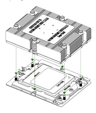
12. Using a diagonal pattern, tighten the six screws down on the heatsink in a clockwise fashion. The heatsink will now be secured and you have finished installing the processor and heatsink onto the motherboard. Repeat this procedure for any remaining CPU sockets on the motherboard.
