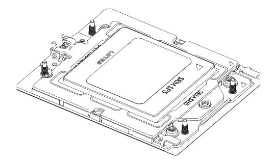
11. After the force frame is secured and the CPU package is in place, now you must install the heatsink to the frame. Lower the heatsink down till it rests securely over the six screw holes on CPU package on the socket frame.
