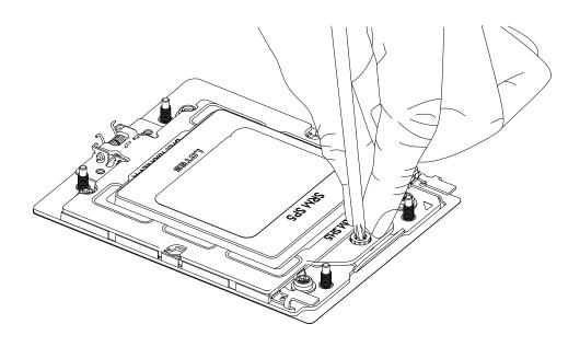
10. Replace and tighten the screws in the same order you removed them. When finished, the force frame will be secure over both the rail frame and CPU package.
