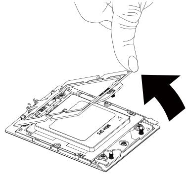
3. Lift the rail frame up by gripping the lift tabs near the front end of the rail frame. While keeping a secure grip of the rail frame, lift it to a position so you can do the next step of removing the external cap.
