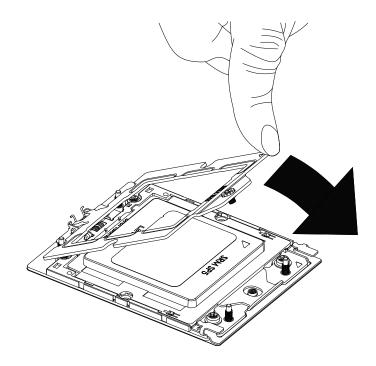
9. The force frame is spring loaded and has to be held in place before it is secured. Important: Use a torque screwdriver, set it at 12.5~15.0 kgf-cm (10.85~13.01 lbf-in) with a Torx T20 screw head bit, to prevent damage to the CPU.
