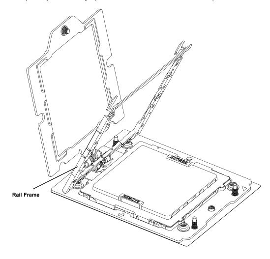
**Warning!** The exposed socket contacts are extremely vulnerable and can be damaged easily. Do not touch or drop objects onto the contacts and be careful removing the PnP cover cap and when placing the rail frame over the socket.
